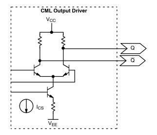
Figure 1. ECL with CML, Current Mode Logic Output Structures
