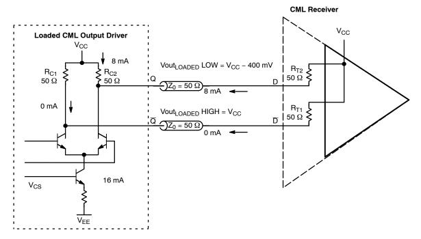
Figure 6. CML Output (with Direct Connect Load Termination of 50  $\Omega$  per line to V<sub>CC</sub>), Currents and Levels (Q LOW,  $\overline{Q}$  HIGH)
