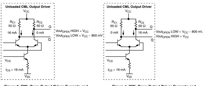
Figure 3. CML Open Output Driver Currents and Levels (Q HIGH, Q LOW)
