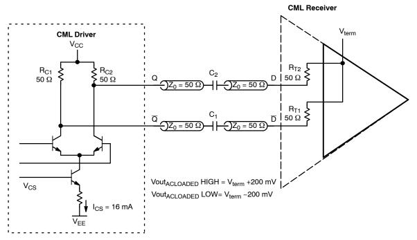
Figure 7. CML Output with Cap Coupling (AC) and Load Termination of 50  $\Omega$  to V<sub>term</sub>
