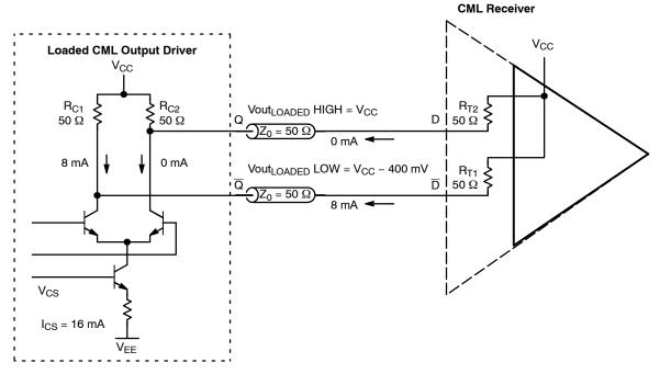
Figure 5. CML Output (with Direct Connect Load Termination of 50  $\Omega$  per line to V<sub>CC</sub>), Currents and Levels (Q HIGH,  $\overline{Q}$  LOW)
