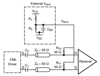
Figure 8. Typical V<sub>term</sub> Supply Divider Network
