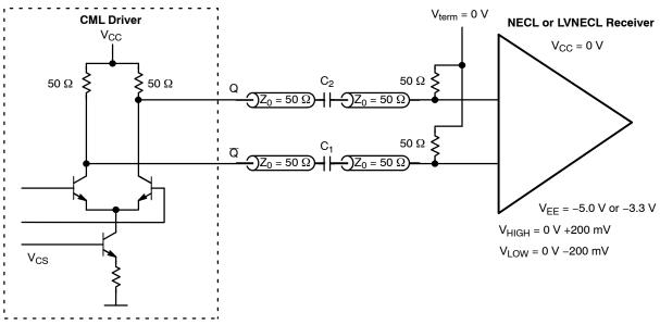
Figure 13. CML to NECL (V<sub>term</sub> = 0 V, V<sub>EE</sub> = -5.0 V or -3.3 V)
