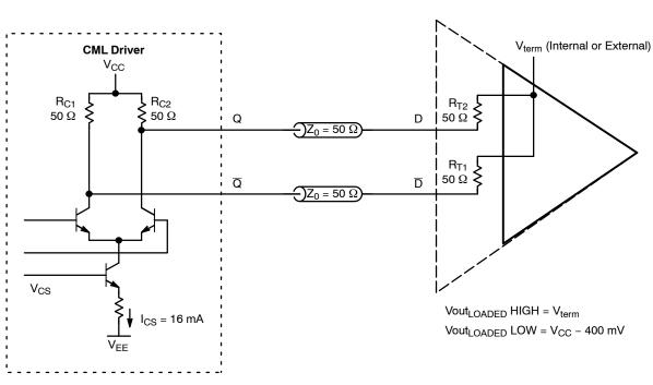
Figure 10. CML Output with Direct (DC) Interconnect and Termination of 50  $\Omega$  to V<sub>term</sub>
