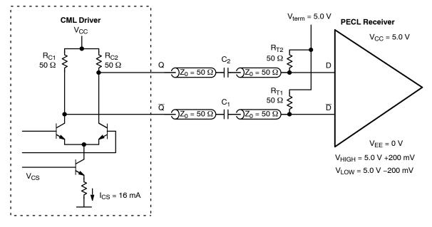
Figure 11. CML to PECL (V<sub>CC</sub> = V<sub>term</sub> = 5.0 V, V<sub>EE</sub> = 0 V)
