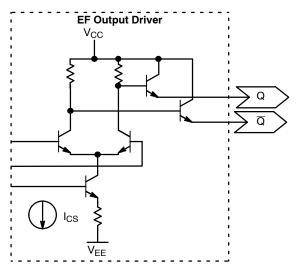
Figure 2. ECL with Emitter Follower Output, Output Structures
